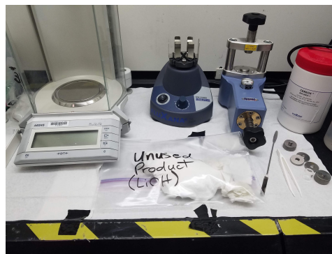
Fig. 1. Equipment used to press the pellets.
