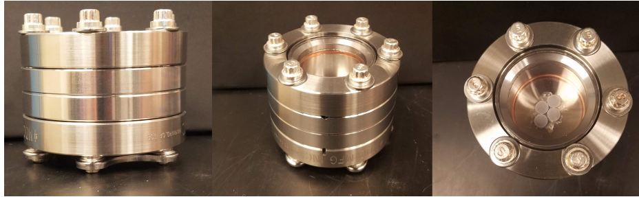
Figure 14. Conflat flange sample cell with UV fused silica viewport. The spacer is used to extend the distance between the focal point of the laser and the glass to avoid damage to the viewport.
