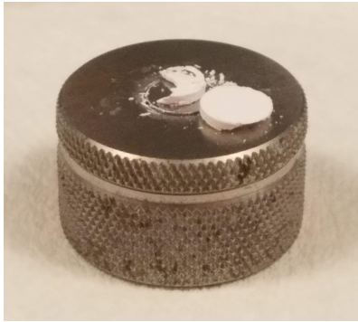
Figure 13. The pure Li_2CO_3 pellet which broke upon removal from the pellet press die on which it is sitting in this figure.
